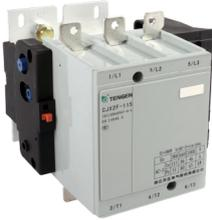
CJX2F series AC contactor (hereinafter referred to as contactor) is mainly used in AC 50Hz or 60Hz circuit with a rated working voltage up to 1000V and with a rated working current up to 800A for remote power-on and power-off of circuit, and can be combined with the appropriate thermal overload relay to form an electromagnetic starter for protection of the circuit that overload may occur.
